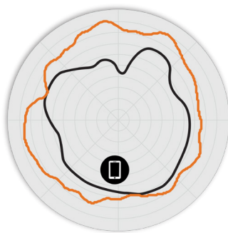
Figure 4. R770 6GHz Azimuth Antenna Patterns
