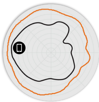
Figure 2. R770 2.4GHz Azimuth Antenna Patterns
